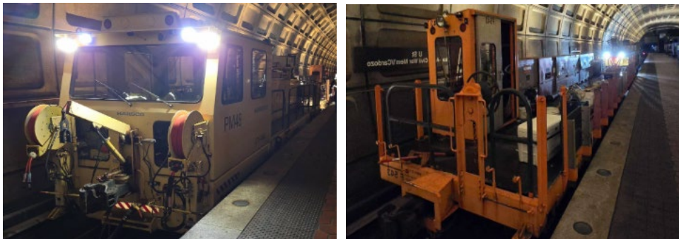
Photo 7 (left): Prime Mover (PM48) white aspect to the front. Photo 8 (right): WMSC Inspectors observed Flatcar 543 red aspects were blinking and therefore their full illumination is not caught in this photo.
