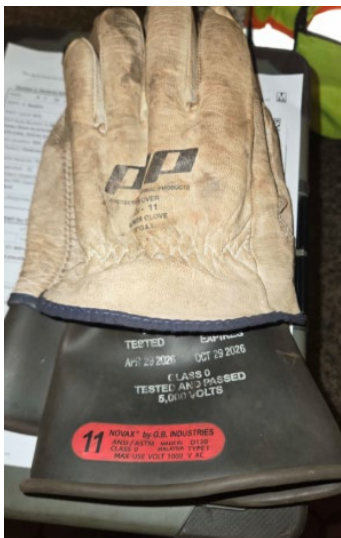
Photo 6: Compliant Class 0 electric gloves used by RWIC.
