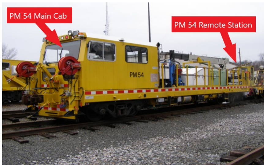
Figure 1 – Depicts Prime Mover (PM) 54, a Plasser PMC-50 Rail Maintenance Machine.
